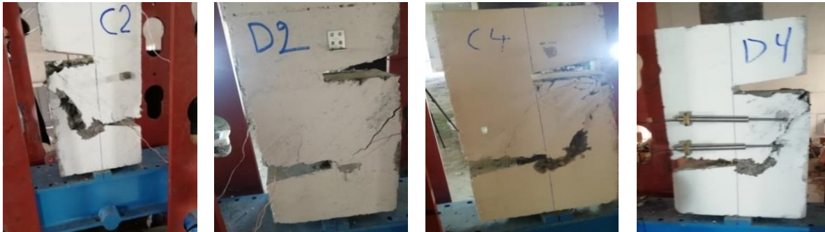
Fig. 6 : Specimens C2, D2, C4 and D4 after failure. (Source: Researcher)
