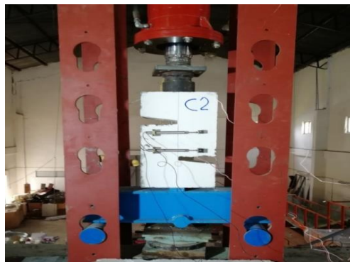
Fig. 4: Instrument and push off specimen that ready for test. (Source: Researcher)
