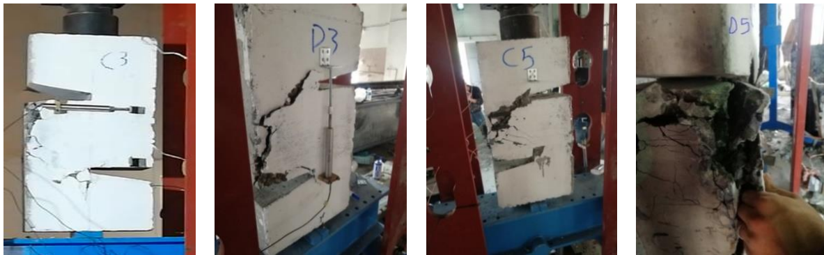
Figure 7 : Specimens C3, D3, C5 and D5 after failure. (Source: Researcher)
